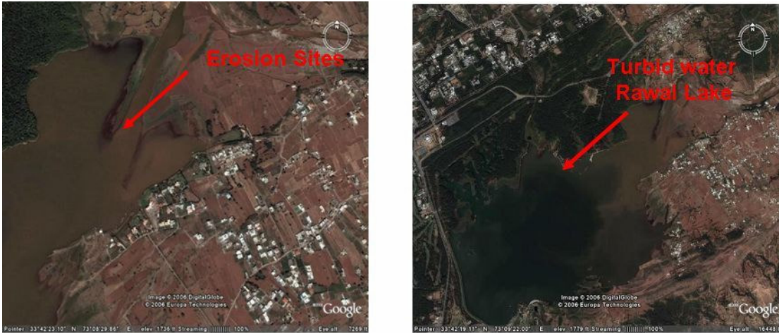
Figure-8: Massive erosion due to intense rains which are causing sediment transport into Rawal Lake – More turbidly with increased levels of contamination
